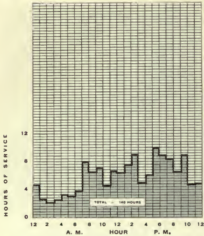
FIG. 427. TRAFFIC DIAGRAM. Locomotive-Hours of Service for the Average Day for Steam Operation in Passenger Transfer Service within Area of Investigation.
